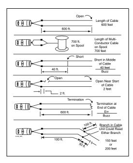
Figure 3. Testing for Length, Shorts, Opens and Terminations
