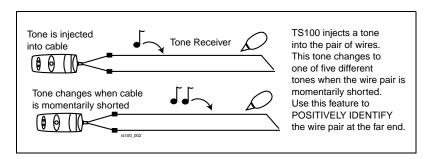
Figure 2. Tone Injection Positive Identification System
