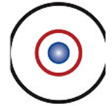
Figure 1. Circular vial with bubble centered in inscribed circle.
